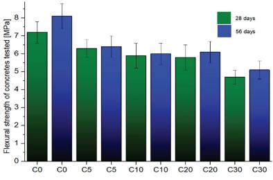
Figure 10. Flexural strength of the concretes tested
