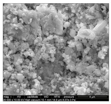
Figure 1. Microstructure of CKD (20,000×)
