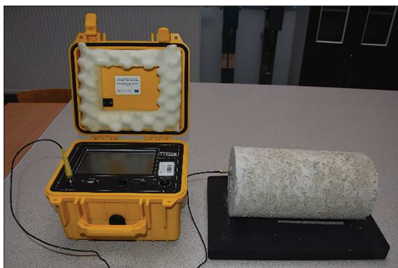
Figure 3. Determination of the dynamic elastic modulus ( E_c, d )
