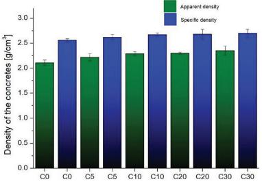
Figure 4. Density of the concretes tested
