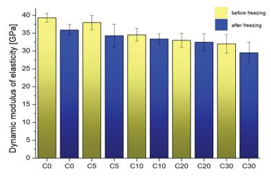
Figure 13. Results of dynamic modulus of elasticity of the concretes tested
