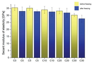
Figure 12. Results of secant modulus of elasticity of the concretes tested
