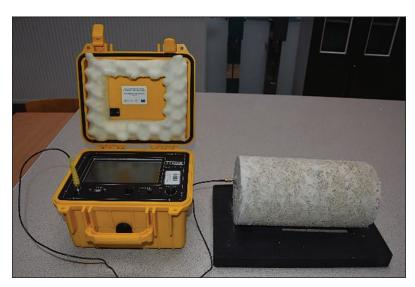
Figure 3. Determination of the dynamic elastic modulus (Ec,d)
