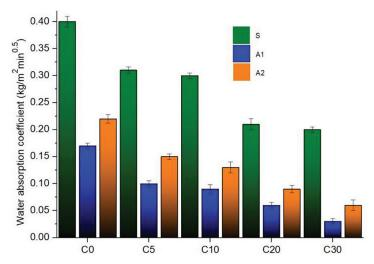
Figure 15. Water absorption coefficient of concrete with CKD
