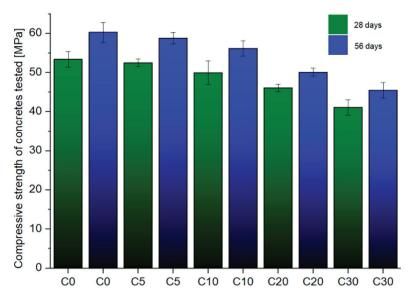
Figure 8. Compressive strength of the concretes tested
