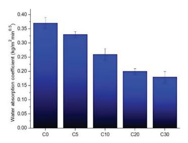
Figure 7. Water absorption coefficient of the concretes tested
