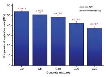
Figure 11. Compressive strength of concrete – results after the frost resistance test
