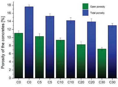
Figure 5. Porosity of the concretes tested
