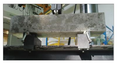
Figure 2. Samples during testing of the flexural tensile strength
