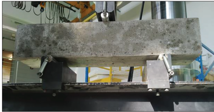
Figure 2. Samples during testing of the flexural tensile strength
